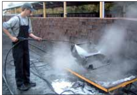
...steam cleaning bogie frames...
